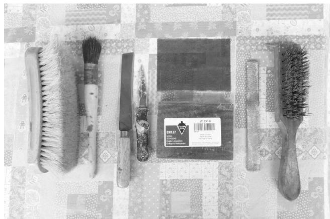
15 The hand cleaning tools of knife, scraper (flat back edge of knife), rasp, griddle paper and brushes.
