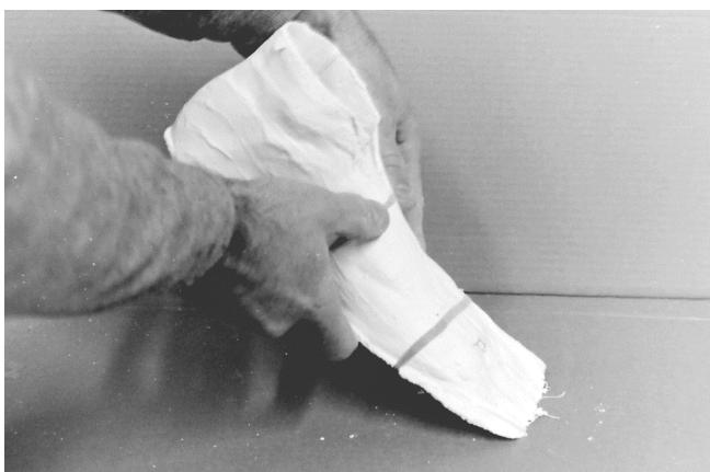
3 The first pour is about 1/3 capacity of the shell. The shell is tilted and shook so the toe area fills without bubbles.
