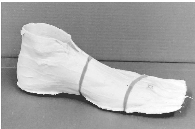
1 The empty shell is best filled about 2 to 4 hours after the casting. When it is dry enough to be hard and yet you can feel a slight touch of moisture, it is ready. Letting the shell sit in the sun or in front of a fan helps it to dry.
