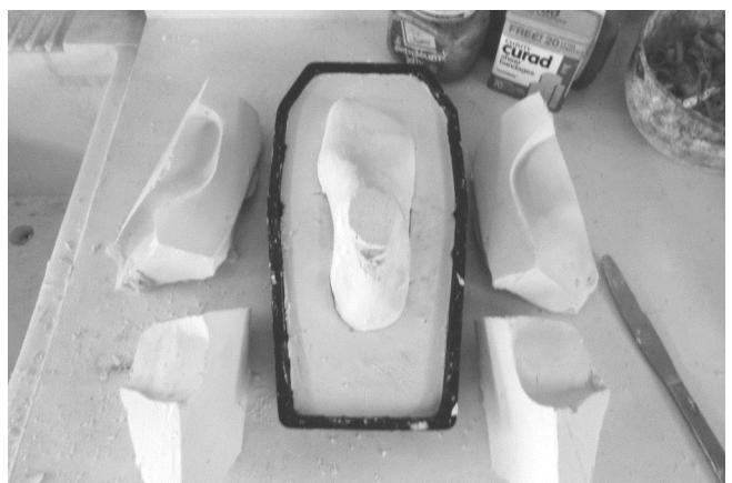
21 The top of negative cast has been separated. The inner cast (which is a cast of a last) is ready to be removed.
