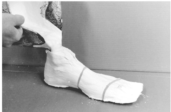
6 The shell is filled as high as possible. The shell is wobbled and the heel lightly tapped on the table top so the plaster settles without air bubbles.
