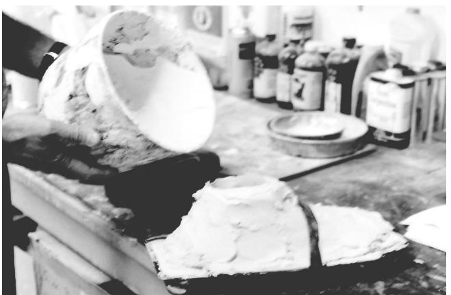
19 The plaster is being poured into the negative cast.
