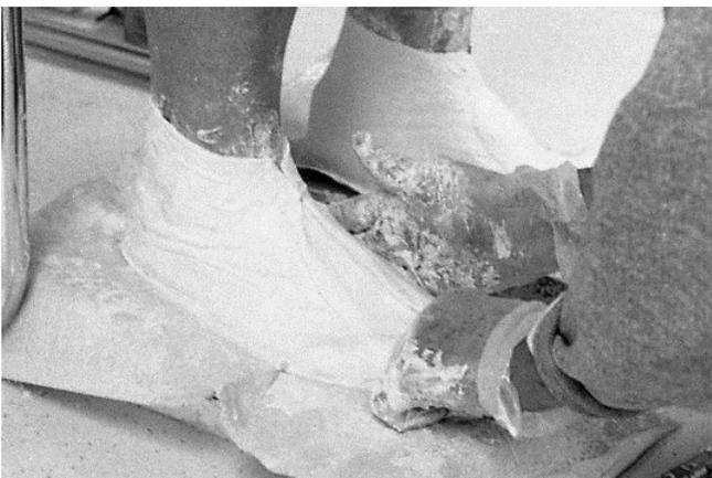
41 The caster is making the upper cast mold to the arch and bottom cast.
