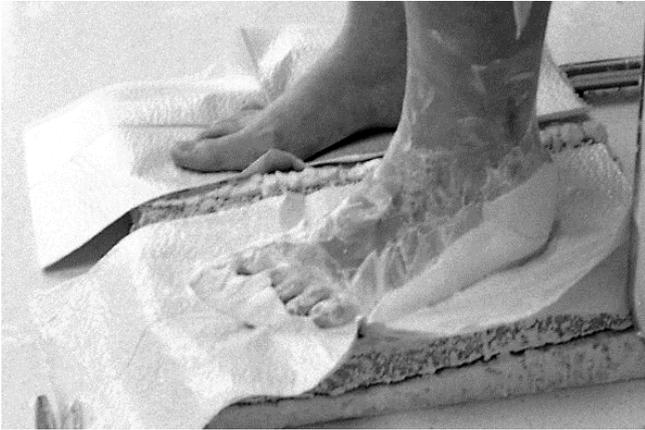
19 The side view of finished bottom of plaster cast. Notice rounded shape at heel. Please look at picture 24 and 25 to see how the arch was molded to fit the customer's foot.
