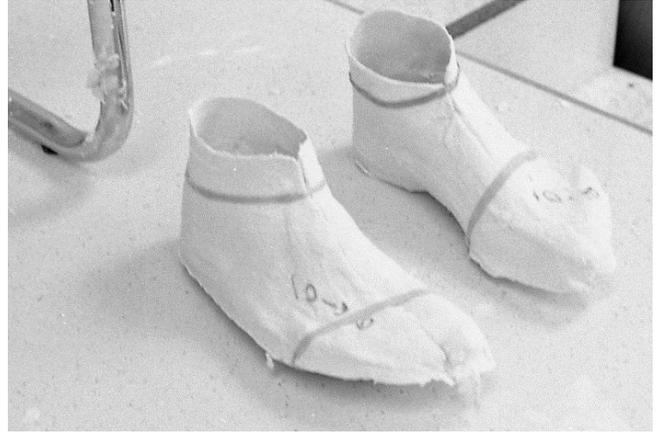
62 Ditto. The excess plaster splints from picture 27 can be used to cover the center seam and bottom under front of toe box so the liquid plaster will not seep out of the seams during the pour up.
