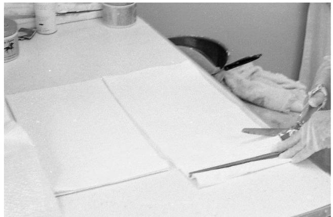
12 The second stack of 5 layers is being cut off the roll.
