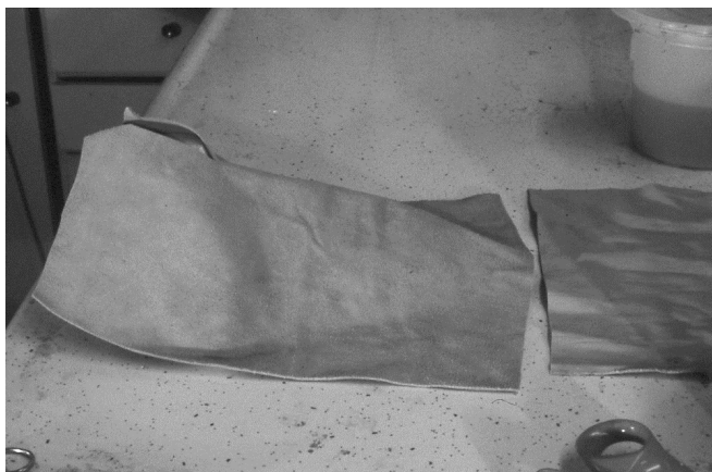
35 A short center cut is made to the top of front leather and stops just before top of shoe design cord.
