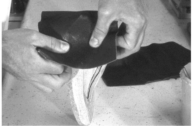
234 Stretching leather to "mold" (conform) it to the shoe.
