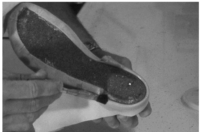
70 Glue is applied to bottom edge of lining leather and Thermocork®.
