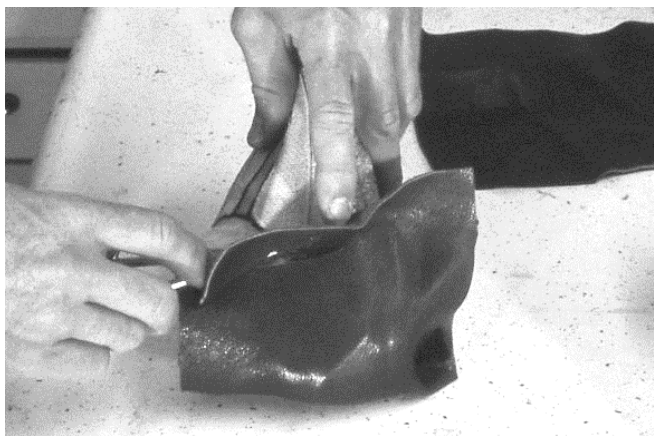
239 Cutting off excess leather on bottom leaving enough to fold over.
