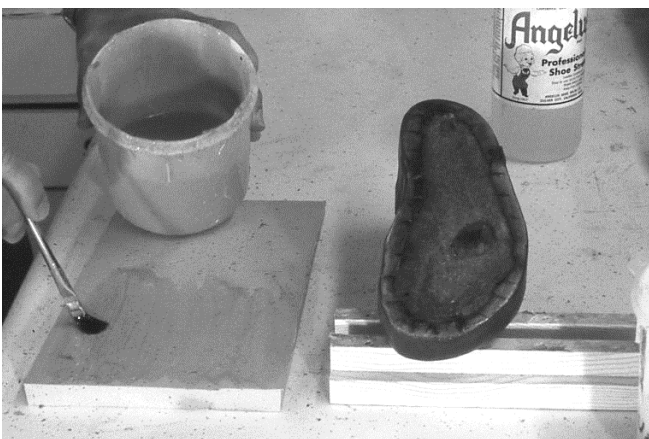
291 Applying glue to mid sole and heel wedge material. This is a special shoe and it used Kingsley Medathane® cushion material which is available from Kingsley Manufacturing company.
