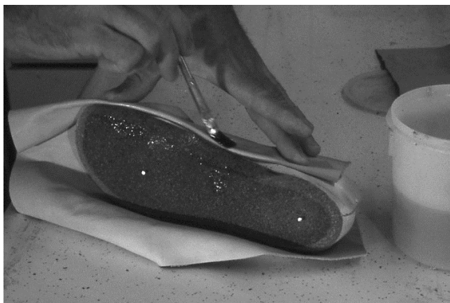
38 Glue is applied to front lining leather.
