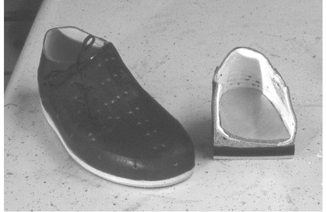
336 Finished shoe is shown next to a cut away showing achievement of individualized molded shoe, which fits contours of the individual foot, as reproduced from a cast of the wearer's foot.
