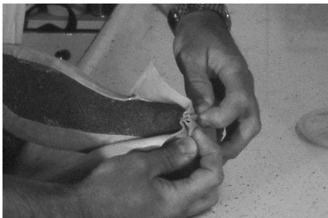
71 Heel lining leather is pulled tight and pressed.
