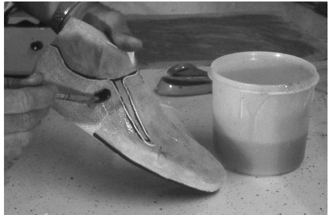
140 Glue is applied to all of shoe except inner part of bottom leather.
