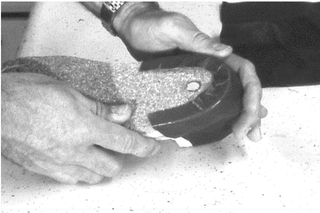
247 Finished result of overlapping heel leather to bottom of shoe.
