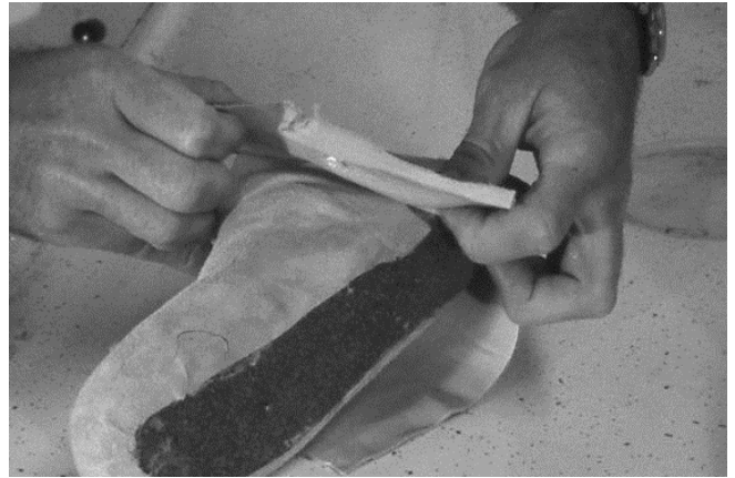
66 Heel lining leather is placed at side seam.
