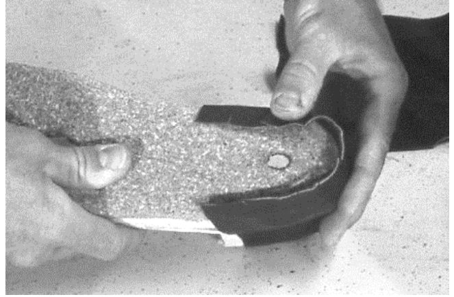
246 Folding over bottom of heel leather.
