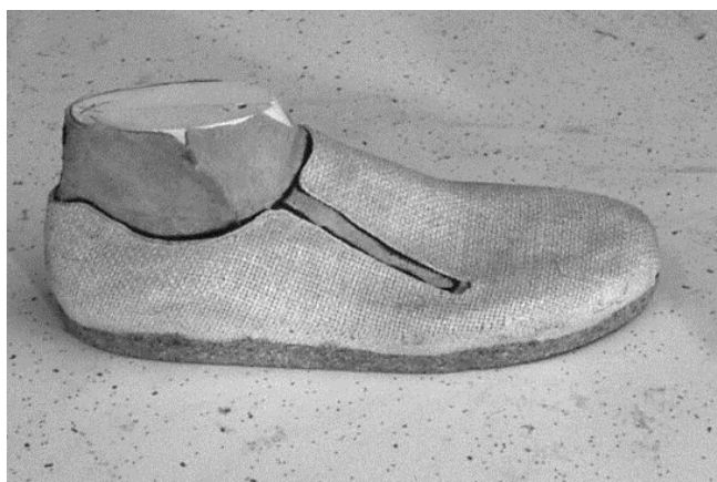
206 View of last with upper materials and "mud" base completed.
