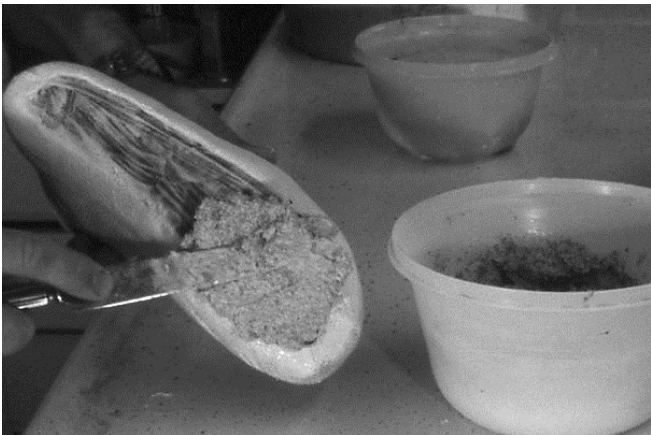
171 "Mud" is applied to bottom of shoe.
