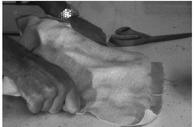
146 Top Monks Cloth is pulled, stretched and pressed into place.
