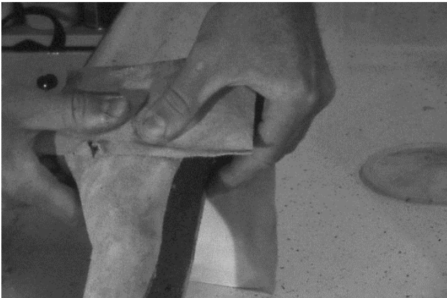
67 Heel lining leather is pressed.
