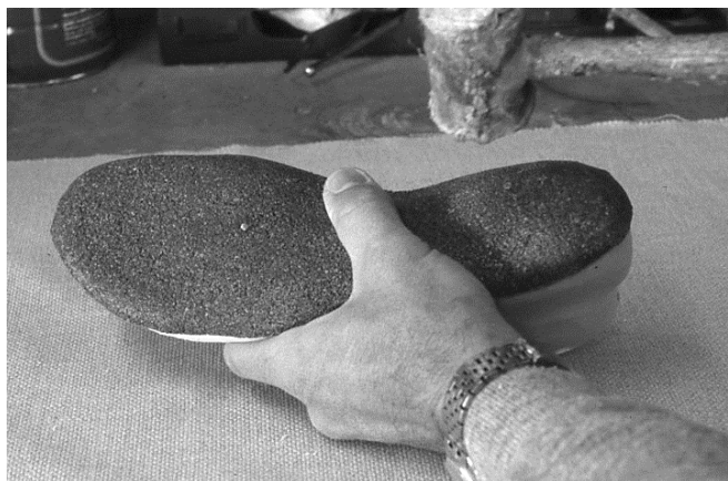
11 Thermocork® is hand tacked to last.
