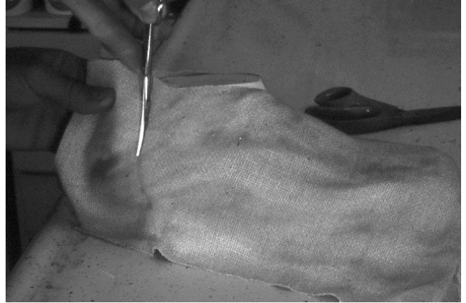
150 Excess can be cut off at back to form a seam with or without overlap.
