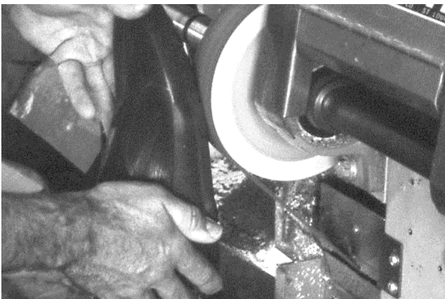
285 Sanding bottom of overlap leather flat and smooth.
