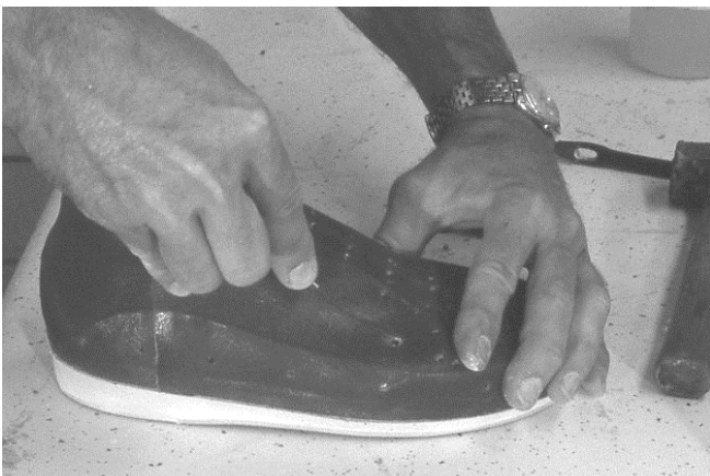
321 Lace opening is cut with single edge razor blade.
