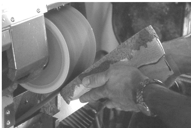
192 The toe to ball is sanded flat (usually).
