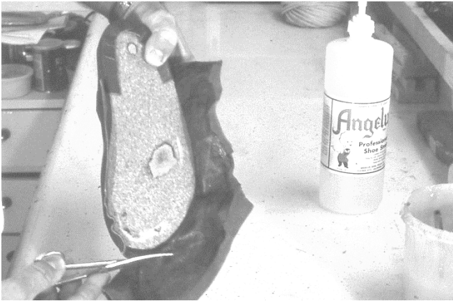
263 Allowing for fold over and cutting off excess from bottom.
