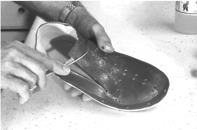
325 Excess leather is cut off above top of shoe.
