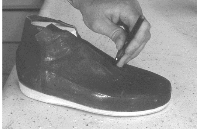
318 Top or cord perforations are punched.
