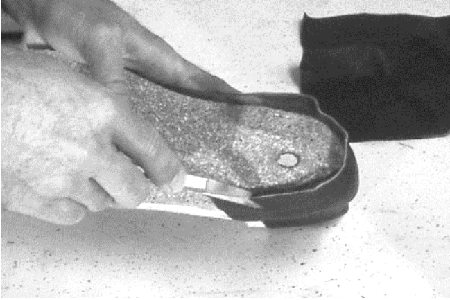
245 Cutting heel leather at bottom.
