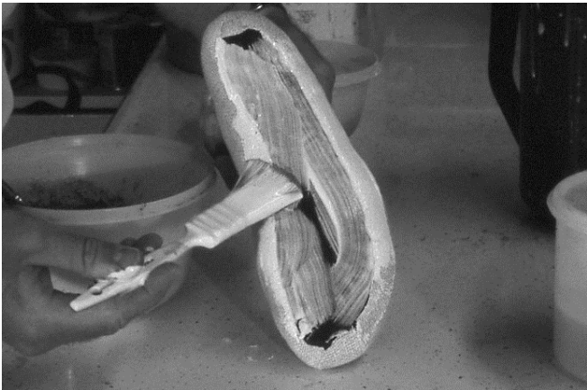
169 Latex is applied to bottom of shoe.
