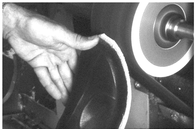
298 Ball to toe is sanded on wheel and/or flat belt sander.
