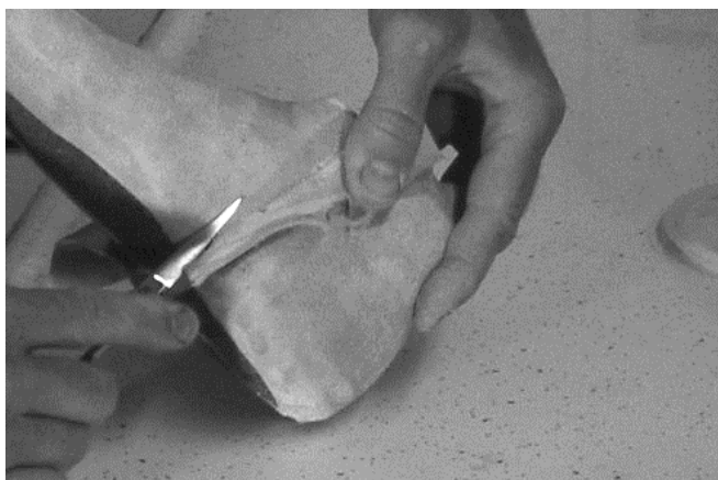
75 Excess lining leather is cut away leaving about 1/2" of side seam overlap.
