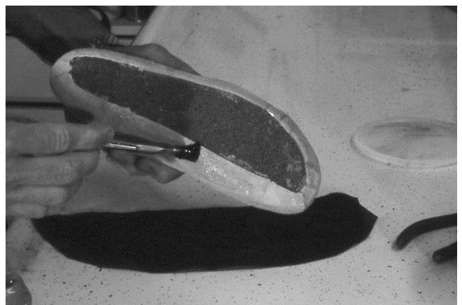
82 Glue is applied to upper lining leather.
