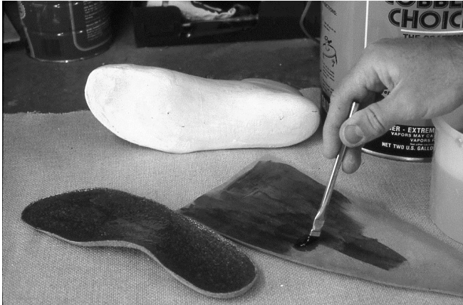
17 Lining leather is turned over and adhesive is applied to bottom of leather and top of Thermocork®.
