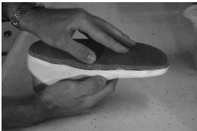
23 Leathered Thermocork® is fitted to last.
