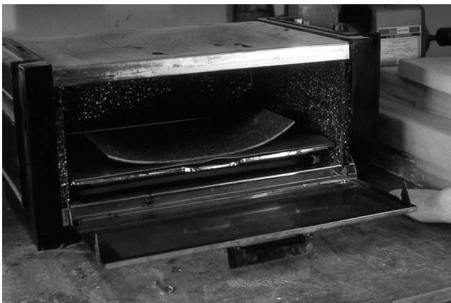
3 The Thermocork® and silicon sheet are placed in oven at about 250 to 275F.
