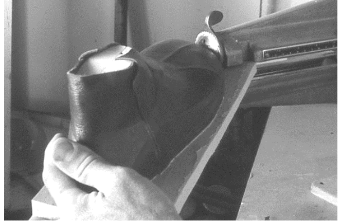
294 Excess material is trimmed away.
