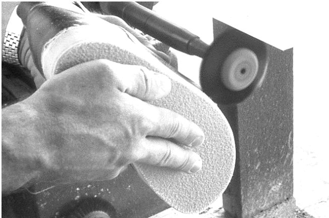
313 A dental lab brush is used to clean leather to mid sole joint area.
