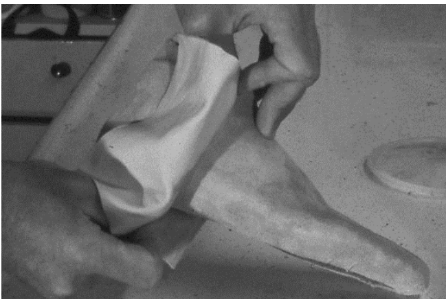
69 Heel lining leather is stretched snugly around back of last, pulled forward to side seam and then pressed.
