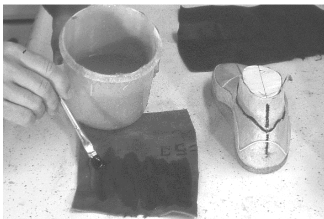
230 Applying glue to under side of heel leather.
