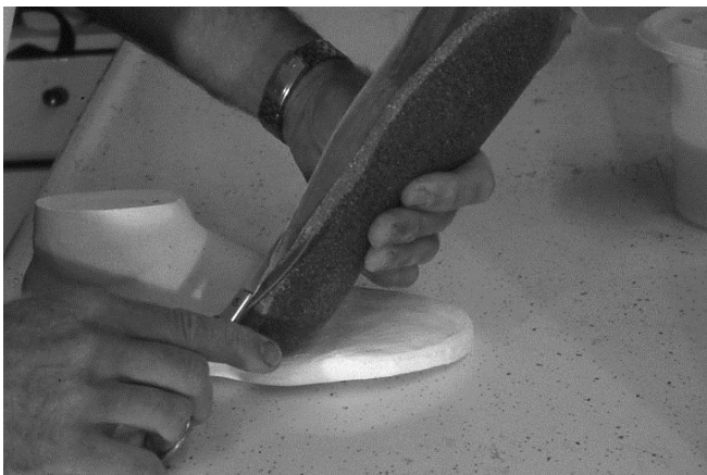
21 Lining leather is trimmed to edge of Thermocork®.
