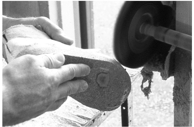
198 The Monks Cloth is wire brushed clean of "mud". Monks Cloth is a stronger fabric than a knitted sock. The weave can be very flexible if the fabric is not "sized".
