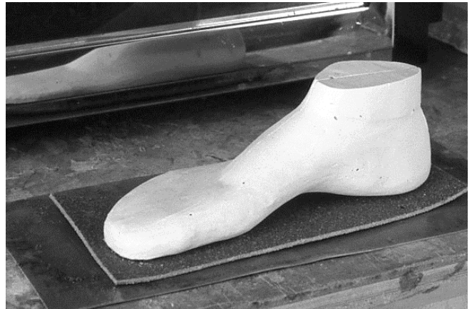
2 The Thermocork® sheet is placed on a silicon sheet which is necessary because of the heat and stickiness of hot Thermocork®.
