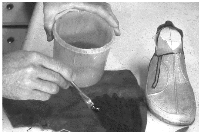
250 Applying glue to underside of front leather.
