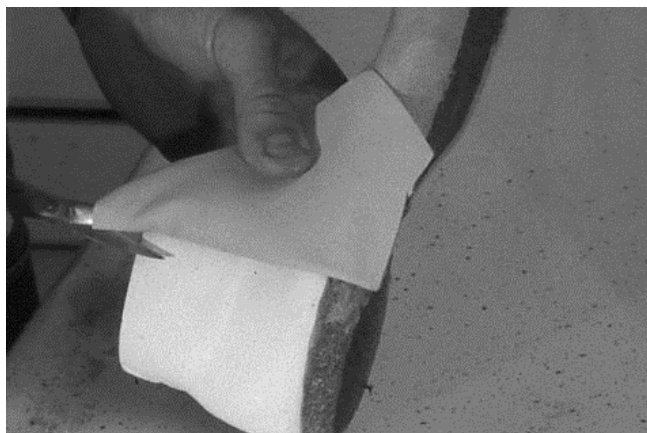
62 Excess lining leather is cut off at desired location of side seam.
