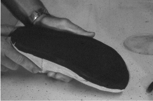
89 View of bottom leather. This bottom leather is really another lining as the leather lined Thermocork® becomes a removable insert.
