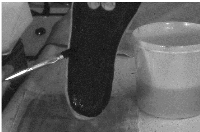
121 Glue is applied around edge of bottom leather.
