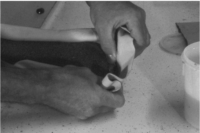
50 Lining leather is stretched and pressed.
