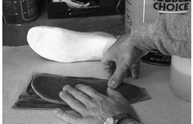
18 Thermocork® is turned upside down and placed on lining leather.
