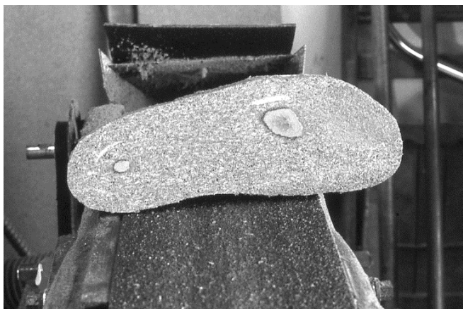
191 The bottom leather has been found. The flat belt sanding has been completed from center of heel to ball of foot.
