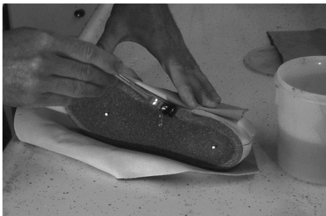
37 Glue is applied to Thermocork®.
