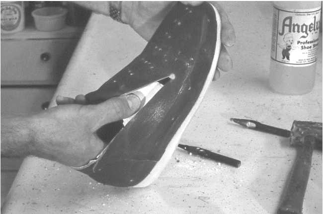
324 Remainder of last is pulled out of shoe.
