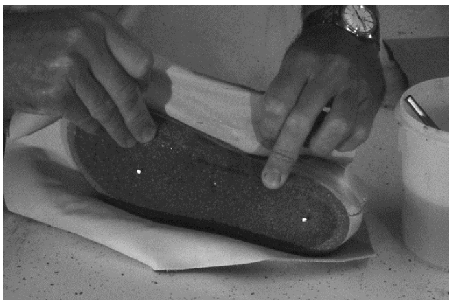
39 Lining leather is stretched into place.
