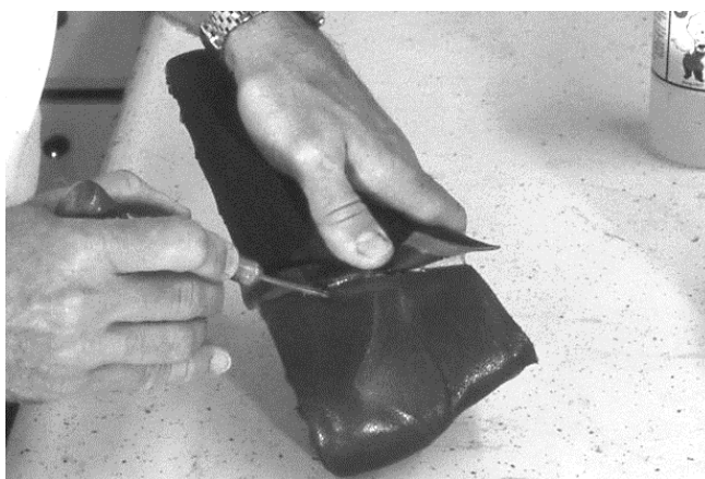
280 Folding back side seam overlap and scratching area to be glued.
