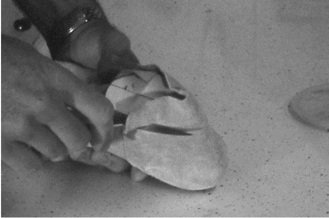
77 Excess lining leather above top of last is cut off.
