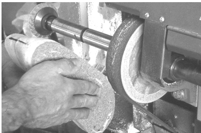
203 Final sanding of outer edge of "mud" base.
