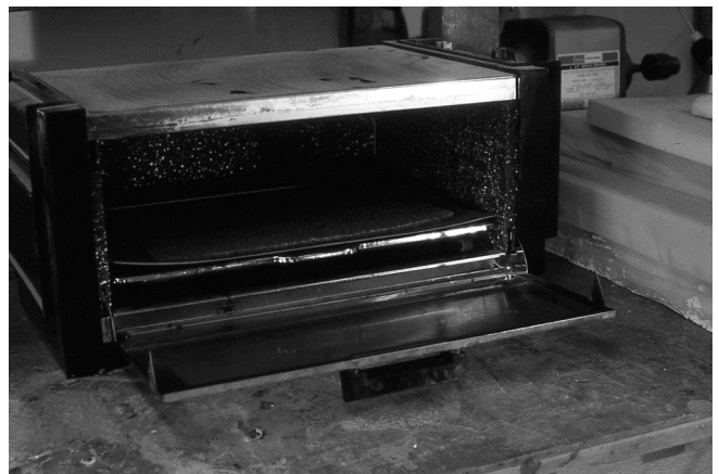
4 The Thermocork® becomes soft and relaxes flat to the silicon sheet.
