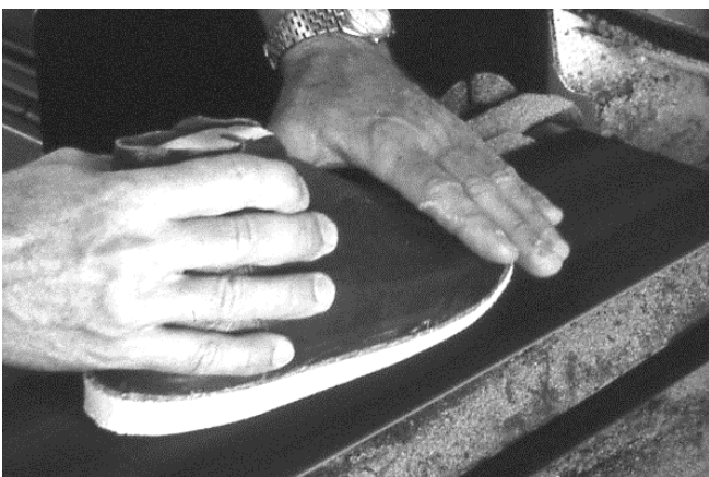
297 Mid sole/heel wedge is sanded to desired taper from heel to ball on flat belt sander.
