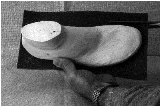
1 A Thermocork® sheet is cut to size for last. This Thermocork® sheet is about 1/8 inch thick.
