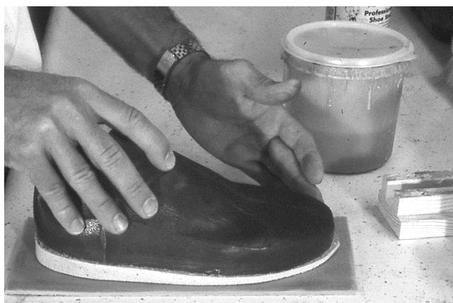
302 Shoe is placed on outer sole.
