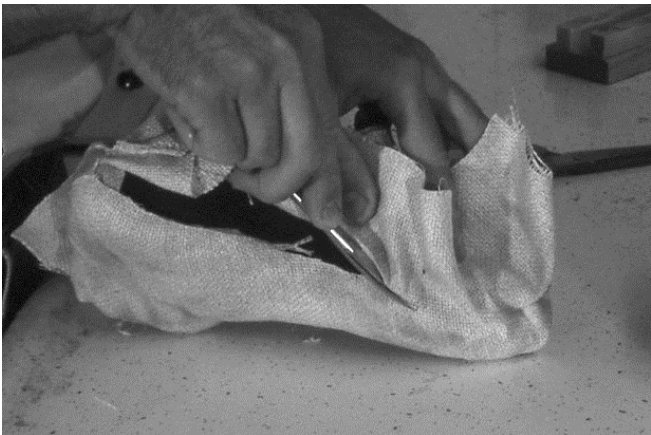
159 The desired overlap is about 1/2" from outside edge of bottom leather. Excess Monks Cloth is cut away.
