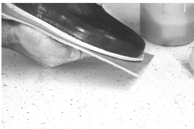
303 Outer sole is pressed onto shoe.
