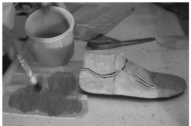
118 Glue is applied to heel Monks Cloth (no sock is necessary for this shoe process).
