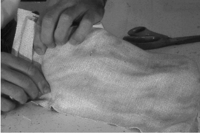
149 Sides are made to fit snugly at back of shoe.
