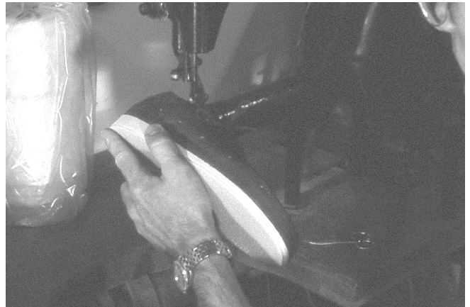
332 Side seam is stitched at top of overlap.
