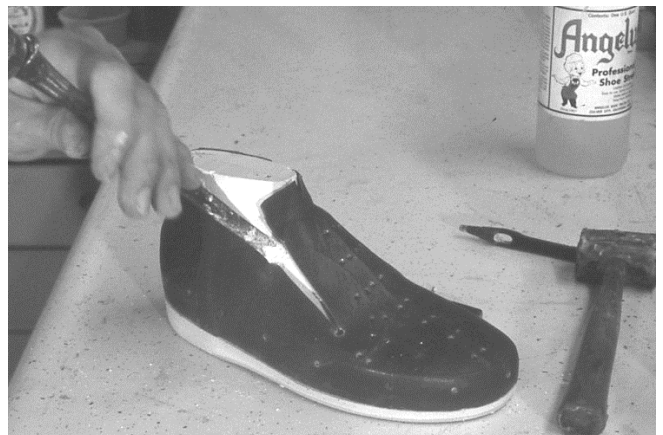
322 Last is broken with a big screwdriver and mallet.
