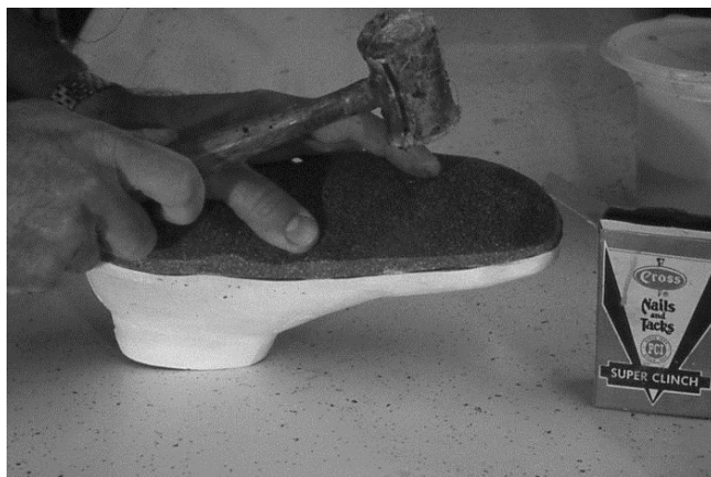
24 Hand tacks are used to secure lined Thermocork® to last.
