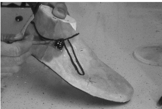
105 Glue is applied to design marking.
