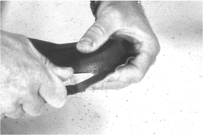
264 Pressing in top leather down to bottom edge.
