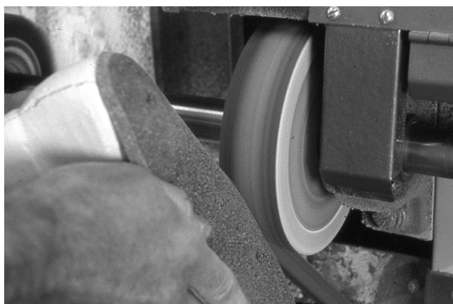
26 The Thermocork® edge is beveled smooth.
