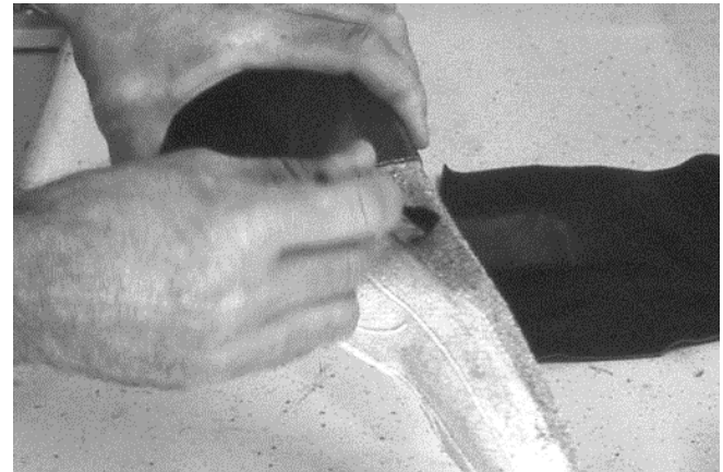
248 Applying glue to front of shoe.
