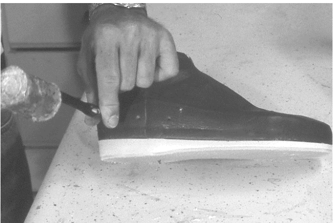
316 Base perforations are punched.
