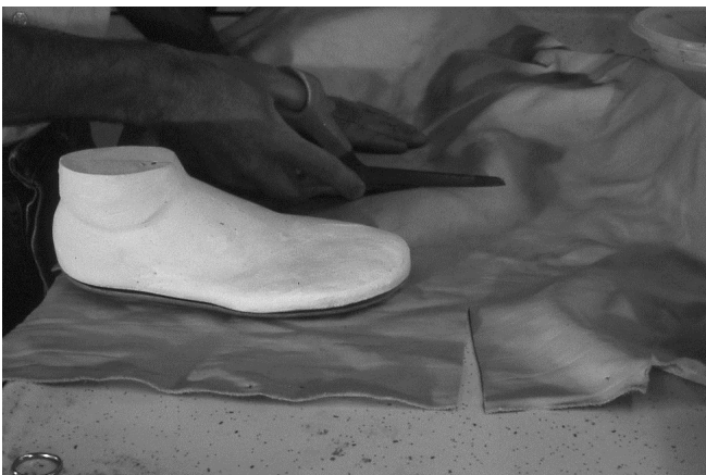
33 Lining leather is cut for front top of shoe.
