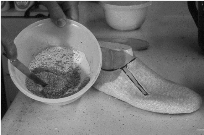
167 Mixing "mud" flour and latex into rubber butter.
